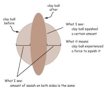
Caption: This sketch shows how a clay ball behaves when it is "squeezed" in a collision. The ball shows the same amount of squish on both sides, so the amount of force is equal. The difference is the forces are in opposite directions.
